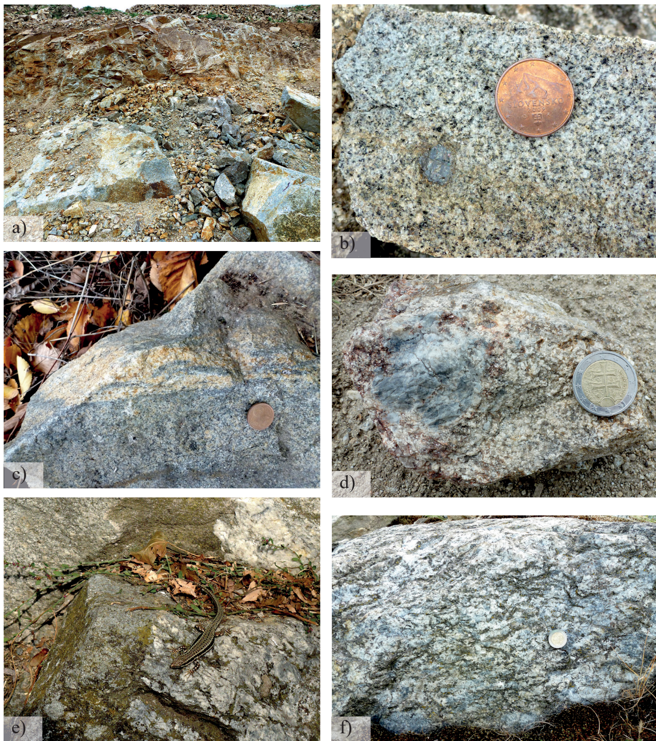
Fig. 1.3 a) characteristic disintegration of granites of the Bratislava Massif (excavation of the northern edge of the Svätý Jur Town); (b) fine-grained biotite granodiorite with biotite phenocryst (ditto); c) penetration of the leucocratic melt into the “basic” granites (Račí potok Brook); d) accumulation of coarse-grained K-feldspars in a leucocratic granite (a fragment at the church in Neštich); e) contact of the three most widespread granite rocks: leucocratic granite (upper left corner), darker two-mica granite (in the middle) in direct contact with pegmatite (rubble dumps SE of altitudinal point Vtáčnik, Bratislava-Vinohrady); (f) diatextite rich in pegmatitoid leucosome (blocks on the ridge between the Fanglovský and Račí potok streams)
