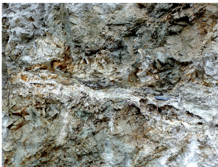
Fig. 1.6 The excavation works in the area of the Bratislava Castle testify to a multiphase neoid tectonic failures of the Castle Cliff; a) brittle deformation, prevailing failure directions dipping to the east; (b) young failure accompanied by the development of a light tectonic clay (scale – geological hammer)
