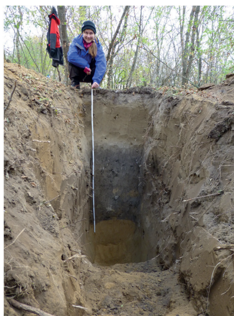
Fig. 3.22 Location Rovinka. Fluvial sands. The white dot indicates the sampling point from which the sediment age was determined by the OSL method at 1,690 \pm 12 BP.
