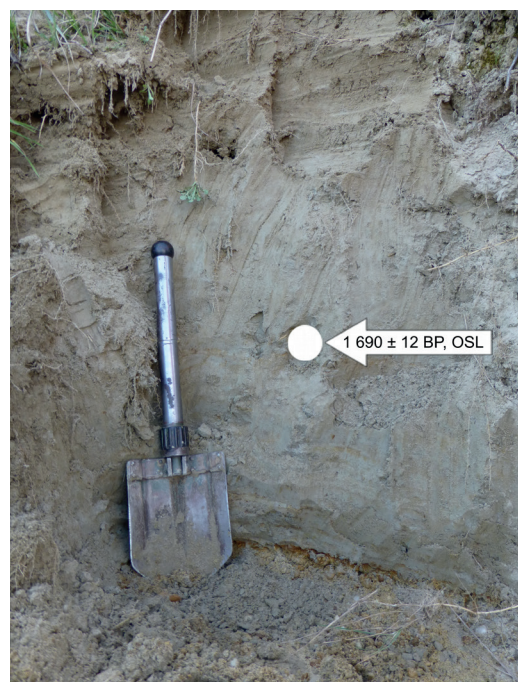
Fig. 3.22 Location Rovinka. Fluvial sands. The white dot indicates the sampling point from which the sediment age was determined by the OSL method at 1,690 \pm 12 BP.
